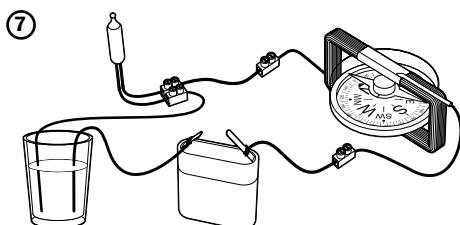
**Test of conductivity of water**
