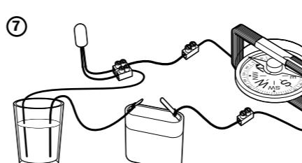
**Test of conductivity of water**
