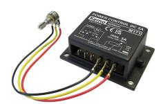
Power control to control direct current loads (motors, lamps, heatings, LEDs with protective resistors, etc.). Electric motors start well also at low revolution speeds because of the employed PWM (pulse width) modulation. Important installation instructions, please note! Modules from serial no. 06022DI (available > 11/2011) can also be connected to a control voltage of 0 - 5 V/DC.
