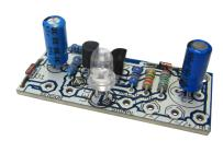
Whenever two bare wires have contact with water, the light emitting diode will light up. The device is suitable to release alarm in case of overflowing rain barrels and gutters. Operating voltage: 9 V/DC. As accessories is available the kit B197 - Relay card 12 V/DC, which could be connected with this kit and could switch through the relay contact other devices (e.g. pumps) up to current consumption of 3 A. Recommended case: G025 - Plastic Case approx. 72 x 50 x 21 mm
