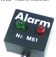
Small alarm monitor with 2 coloured LED's which quick and alternately flash in a special brightness.
